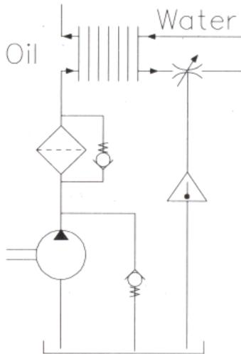
To be able to control lubrication, viscosity needs to be kept constant, meaning that output temperature has to be very accurate.
