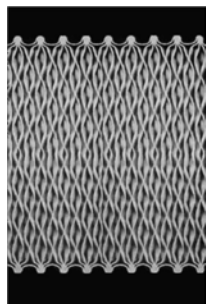
Detail of welded plate packet. TIG welding is used. The welded plate packet is tighten in stainless steel or painted carbon steel frame.
