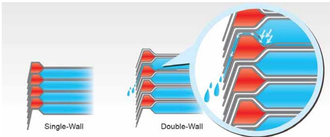
Once a leakage occurs, liquid will seep throughout the air gap to the atmosphere as indication of internal leakage
