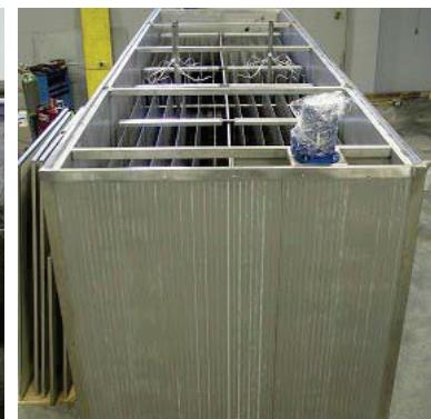
T COIL series heat exchangers are very versatile and efficient prime heat exchangers, which are made with simple and efficient methods: two metal sheets are welded together and, by means of spot welding, they are inflated through high pressure to obtain internal channels that create a series of passages for the heat transfer fluid.
