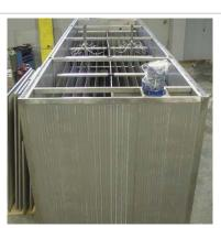
T COIL series heat exchangers are very versatile and efficient prime heat exchangers, which are made with simple and efficient methods: two metal sheets are welded together and, by means of spot welding, they are inflated through high pressure to obtain internal channels that create a series of passages for the heat transfer fluid.
