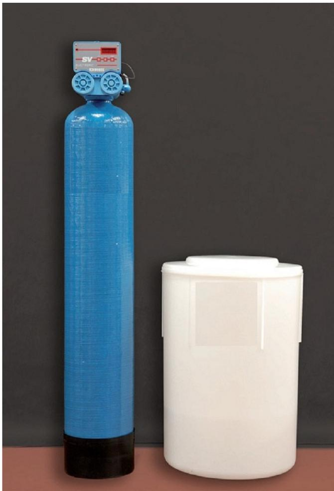
Vessel in fiberglass reinforced polyester resin, exchange ionic resins for softening, with high exchange capacity and specific for drinking water, brine tank in shock resistant plastic material, control valve 5-cycles working (backwash, brine draw and purge, rinse, brine refill, service) with visual function and pre-set mode.
