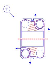
1.1. Leakage through the leakage vent:
